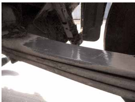
Example of leaf spring surface prepared for application of adhesive tape.
